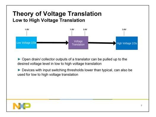
Open drain outputs and low input switching thresholds of CMOS devices are common techniques for low to high voltage translation.
