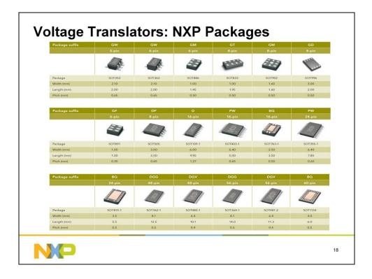
Standard SO, SSOP and TSSOP packages are offered in addition to innovative smaller leadless MicroPak and DQFN packages for voltage translators from NXP. Packages from NXP are RoHS compliant with no lead and are also dark green with no halogen and antimony oxides for better safer environment.
