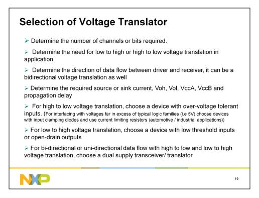
The slide provides helpful hints for selection of a right voltage translator in a system. Determination of number of channels, direction of data flow, translation voltage and current levels and required propagation delay are critical in selection of right voltage translator. With NXP's broad voltage translation portfolio, right voltage translator is always available for any application with specific operating requirements.
