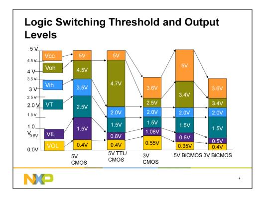
Input switching threshold and output voltage levels for 5V/3V CMOS, mixed CMOS/TTL and BiCMOS logic families are shown here. High level output voltage (Voh) of driver device must be higher than high level input threshold voltage (Vih) of receiver device and the low level output voltage (Vol) of driver must be lower than low level input threshold voltage (Vil) of receiver for proper working of CMOS devices.
