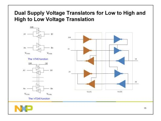
These are the devices with two supply voltages and different voltage ranges. These translators can be used for uni or bidirectional voltage level translation. Some bidirectional voltage translators have a 'DIR' pin to control the direction of data while others have 'DIR" and 'Output Enable' pins for tristating the outputs and save power. Output enable control is available in 245 functions. Low to high as well as high to low voltage translation can be done with these devices.
