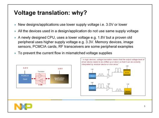
Voltage translation is required to ensure that devices operating at different supply voltages in a system are able to work with each other without any damaging current flow and signal loss.
