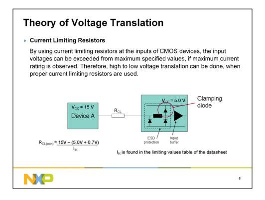
Use of current limiting resistors in CMOS devices for high to low voltage translation is explained in this slide. Value of required current limiting resistor can be calculated by using Vcc values of driver and receiver devices and allowed input clamping current for reciever as shown here.
