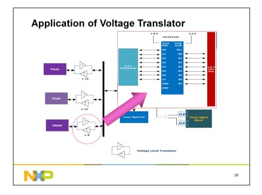
An 8 bit, dual supply voltage level translator is used to translate the voltage signal levels from 1.8V CPU bus to 3.3V memory and vice versa.
