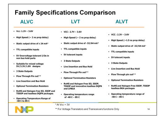
ALVC logic is a high speed version of LVC logic with supply voltage range of 1.2V to 3.6V. LVT and ALVT are BiCMOS logic devices with drive currents as high as 64mA, suitable for high load applications. Outputs of LVT and ALVT devices can be tristated with output enable control and during power up and power down. Also the inputs of these devices are over voltage tolerant. These features provide an additional level of live insertion for LVT and ALVT voltage translators.
