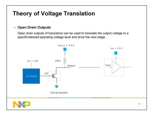
A pull up resister can be used with the open drain outputs of standard logic functions to implement the low to high voltage translation and drive the next device as shown in this slide.
