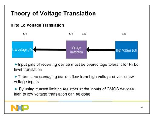
If inputs of receiving device are over supply voltage tolerant, they can accept the input signals which are higher than the supply voltage. Since the outputs of such devices are referenced to Vcc, high to low voltage translation becomes possible. Use of current limiting resistors with CMOS devices which have diodes between inputs and Vcc is another technique for high to low voltage translation.
