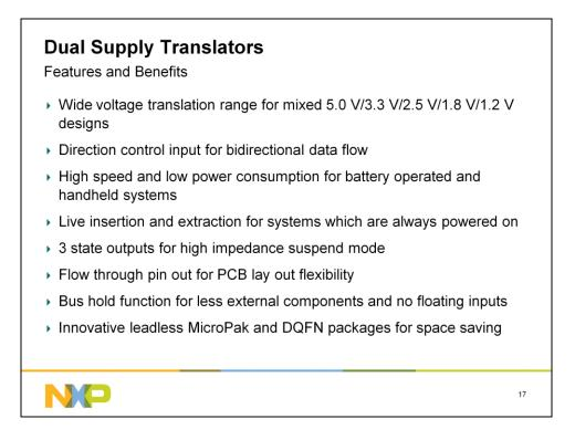
Dual supply translators are available with various unique features that make them suitable for many different applications. Bidirectional data flow, flow through pin out, bus hold and live insertion are some of these features.
