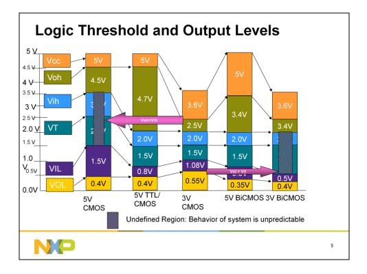
However, if Voh of driver is lower than Vih of receiver and/or Vol of driver is higher than Vil of receiver, the system behavior becomes unpredictable as shown in this slide. Therefore, it is necessary to match the input switching thresholds of receiver with output voltage levels of driver in a mixed voltage system.
