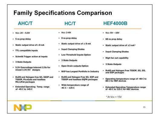
For high to low voltage translation HC/T, AHC/T and HEF4000B logic families offer different logic functions with over supply voltage tolerant inputs and built in Schmitt trigger for slower inputs. With TTL compatible inputs, some level of low to high voltage translation can also be achieved. Wide operating temperature range of -55C to 150C makes these devices ideal for use in systems designed for harsh weather conditions as well.
